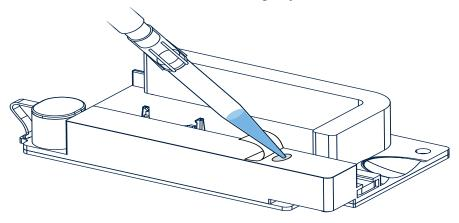
**Note.** Incorrect addition of the Elution Buffer into the X8 Cartridge can result in little or no elution of the purified nucleic acid.
