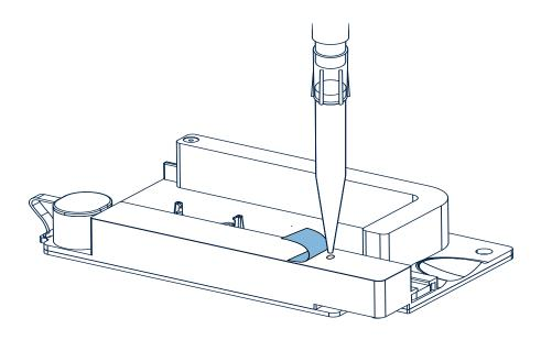
3. Carefully aspirate 150  $\mu$ L of the DNA Elution Buffer (PN. X8-EB1), ensuring there are no air bubbles.
